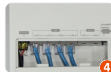
4.Connect the Ethernet port of the PoE camera to the downlink port of the PoE switch.
