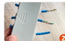
2.Insert the Ethernet cable through the cable entry.
