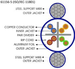
CAT6 cables reduce crosstalk and system noise. The superior insulation around the 23AWG copper wires attributes to the increase performance. They cable transmit data at 1000Mbps (1Gigabit per second) with a frequency of 100MHz and suitable for 10BASE -T, 100BASETX fast ethernet and 1000BASE-T / 1000BASE-TX (Gigabit Ethernet)
